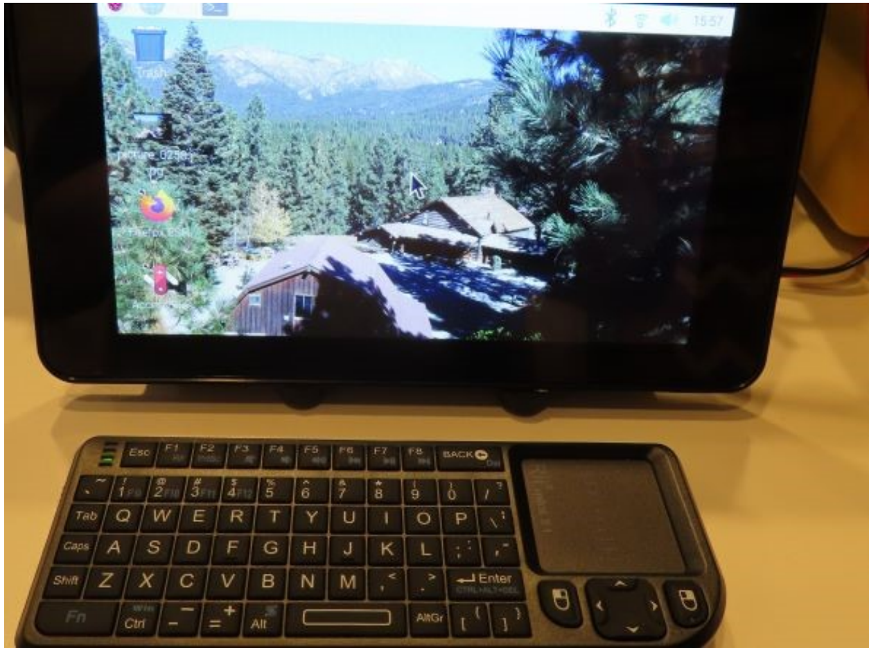
RPI 4B mounted in an RPI display with mouse and keyboard.
