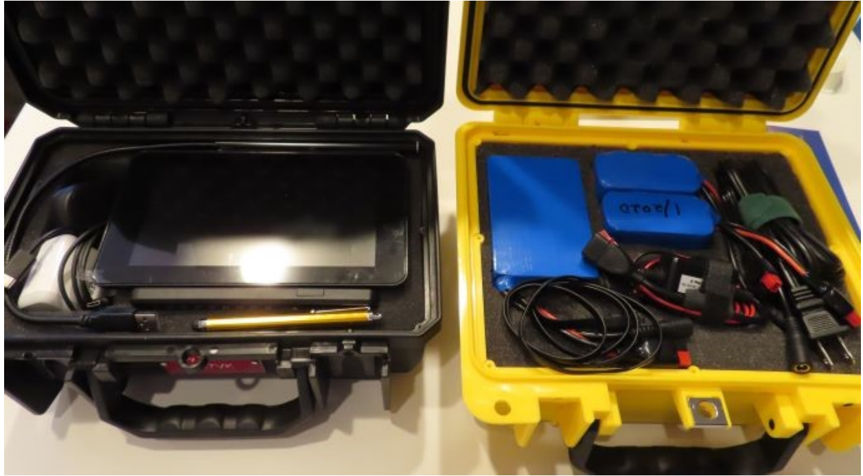
RPI in case and power pack for both Raspberries. Each RPI is powered by step-down transformers purchased at "PowerWerx.com." Everything else was purchased on Amazon.
