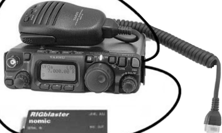
**TRANSMIT AUDIO:** Supplied 3.5 mm, 1/8" stereo phone plug audio cord from computer's headphone\* output to RIGblaster's audio in.
