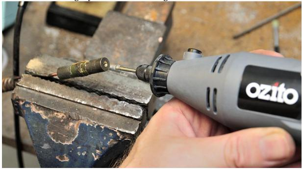
Above: A "Dremel" type tool, and this bit, was perfect for cleaning the gunk out of all the antenna's brass joining sections.
