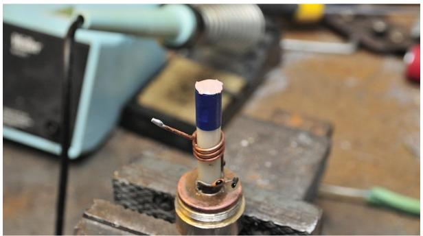
Above: Using electrical tape to form the sides, a small amount of 2-part automotive bog was used to fill in the bit that melted off!
