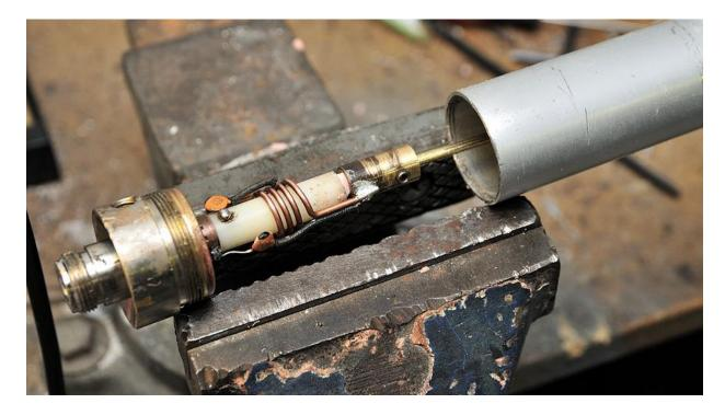
Unfortunately I applied too much heat (using a large Weller 700F tip), and the end of the nylon former (on which the brass end/joiner screwed on to) became soft and melted out of shape.
