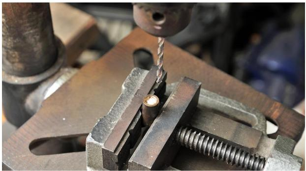
Above: The remaining nylon (I think it's nylon?) was drilled/scraped out of the brass piece.
