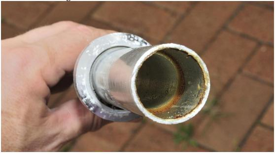
Above: The fibreglass radome section is glued into the base aluminum tube.
