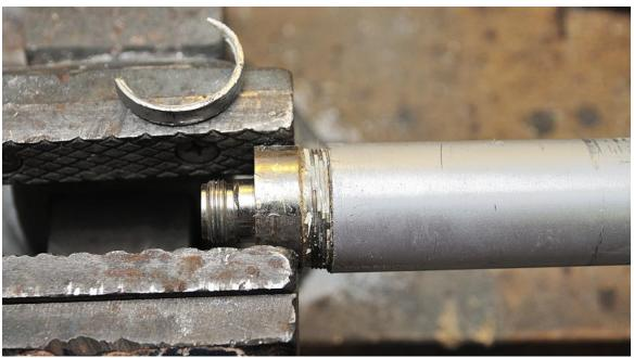
Above: The brass end with the N connector screws into the aluminum base tube section.
