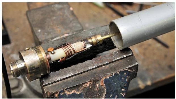
Above: This is what's inside! A tapped coil, a 10pF ceramic in series with coax inner, and a 1.5pF shunt.
