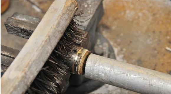
Above: Use a wire brush to remove the adhesive and gunk off the threaded end. Ally tube in place to protect the other components whilst brushing.
